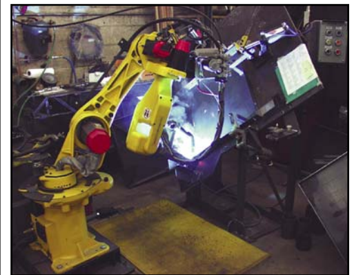
Pictured above is the new robot welding the corners of a landing.
